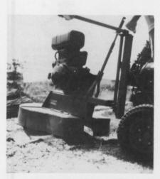
Heckendorn Mfg. now has an 8 hp stump remover that quickly reduces most stumps to an easily removed pile of fine chips, leaving a clean depression ready for grass plugging. The steel cutter disc is 12 in. by 1/2 in, with four hardened carbide teeth. Depth of cut on each pass of the disc can be regulated by a hand screw adjustment. The Heckendorn Stump Remover can be mounted using conventional universal supports.
