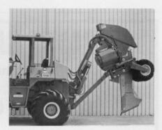
A new heavy duty vibratory plow module, the vp-100, is now available from Ditch Witch for use with the Ditch Witch model R-100 Modularmatic 100 hp class vehicle. Special hydraulic title on frame allows adjustment for vertical plowing and increased stability on slopes.
