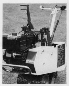
A new belt guide is featured on 1977 model Jr. Sod Cutters under production at Ryan. The guide reportedly is designed to prevent drive belts from slipping off the pulleys and being damaged.
