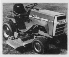
Massey-Ferguson has expanded its line to include the new MF 1655 garden tractor powered by a twocylinder, 16 hp, 40.3 cu. in. engine. Standard equipment includes head and tail lights, Timken wheel bearings, 31/2 gal. fuel tank, and guage wheel adjustment for mower weight. The MF 1655 offers a 12 volt battery and disc braking on the transaxle to supplement hydrostatic braking within the transmission.
