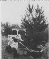
to the manufacturer, include an ability to be attached or detached in minutes, quick-couple to available hydraulic-accessory circuits, operate at maximum without outriggers or other accessories, exert more than four tons of pressure to dig in the hardest earth, ball a tree for basket or burlap sacking and load or unload trees from truck-bed heights.
