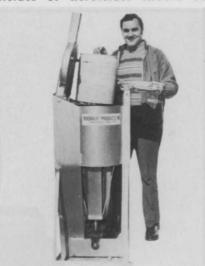
crushed, according to the National Agricultural Chemicals Association. Richway Products is now manufacturing a can crusher that crushes all kinds of metal containers. The unit operates hydraulically and flattens a fivegallon can down to about two inches in a single stroke.
