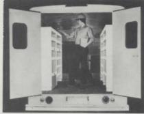
steel back riveted in place for maximum rigidity and convenience. Bin dividers are optional and all shelves install singly or stack.
