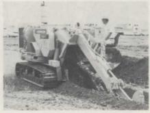
trenching machine now offers the Detroit 4-53 diesel engine as an additional option. Two major improvements are incorporated into the new machine — greater track clearance and enclosure of the final trencher drive in an oil-filled case.
