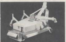
by Sun-Mastr Corp. The unit was specifically designed for use with smaller tractors in the 16 to 30 PTO horsepower range. The unit also features drop-design blades.
