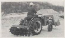
tors, according to the manufacturer, Engineering Products Co. The harrow and other rear-mounted tools are attached in minutes by means of a standard three-point hitch. It is not necessary to remove front-mounted tools when using rear-mounted tools.
