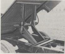
truck hoist. Patterned after its heavy-duty predecessor, the unit nests within the frame without raising the bed or decreasing road clearance. With a three-ton capacity rating, the manufacturer claims it can lift as much as the truck is built to haul.
