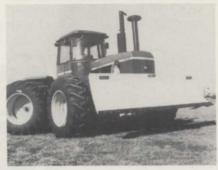
blade with the new mounting kit available from Waldon, Inc. The unit features solid mounting to the tractor frame, direct hydraulic cylinder hook-up, reversible and replaceable cutting edge and dual cylinder operation.
