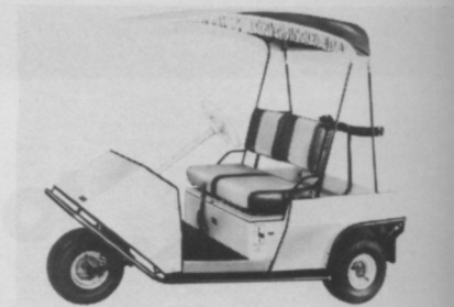
WESTINGHOUSE makes a three-wheel electric that weighs 965 pounds and a four-wheel that weighs 1,030 pounds.
