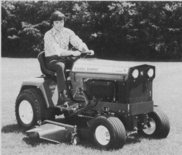
D-250 with 60 in. mid-mounted rotary mower.
