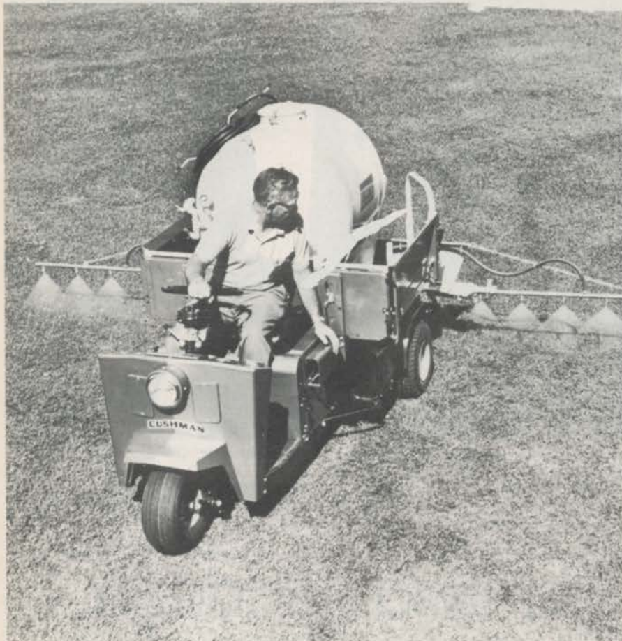
CUSHMAN's Turf-Truckster is equipped with an optional power take-off package, PTO extension shaft and sprayer rig.
