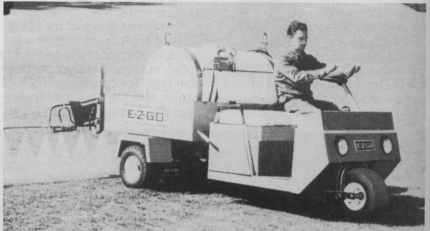
THIS IS the GT-7 Truck from E-Z-GO, re-introduced this year. It's powered by a 20 hp ONAN and has a rated payload of 1,500 pounds.
