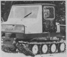
BOMBI: This new multi-terrain personnel carrier, smallest industrial tracked vehicle made by Bombardier Limited, has an enclosed steel cab designed to meet OSHA rollover protective standards. The three-man carrier can be used in snow, swampland, and other offroad areas.
