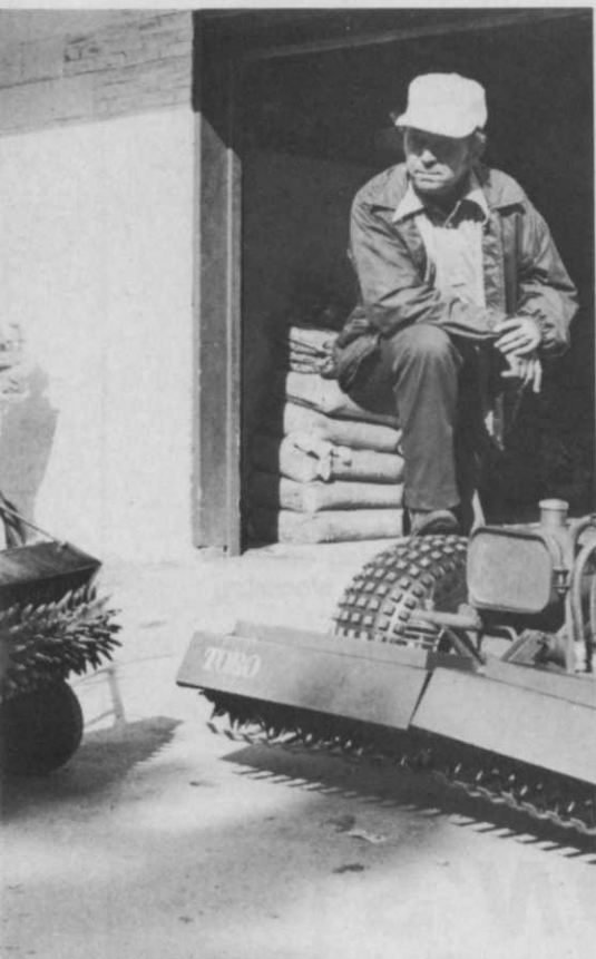
Santoianni compares his recently-obtained Sandpro with the smaller machine his crew formerly used to rake sandtraps. The bigger machine reduced the time requirement by more than half, he says.
