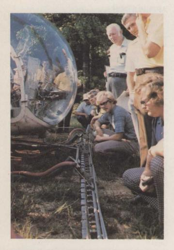
Another factor contributing to his best-ever season Hill attributes to the use of a boom and nozzle arrangement manufactured by Amchem Products, Inc., Ambler, Pennsylvania. The boom, called the Microfoil, is hardly a newcomer to the helicopter application field. "Tex" Waldrum of Amchem's Mechanical Research and Development Division pioneered the boom in 1967. Since that time, the boom has been equipped with a variety of nozzle configurations and ending, at present, with the .060 nozzle.
