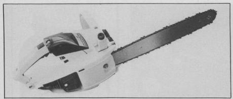
MINI: A new lightweight chain saw introduced by Pioneer weighs about 6.6 lbs. without attachments and has a 2.2-cubic-inch engine. The manufacturer says other features include die-cast magnesium construction, a self-cleaning automatic oiler with manual override, a Tillotson carburetor, and a standard 12-in. sprocket nose bar.
