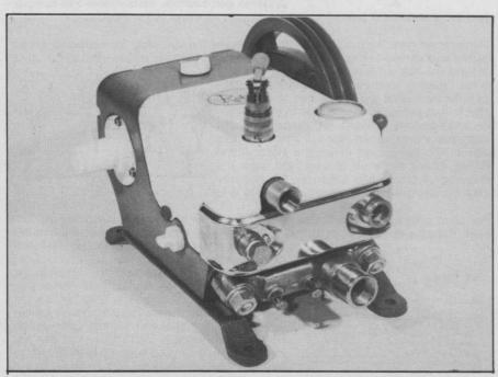
PCO PUMP: This unit is available in five models from 2 to 30 GPM at 500 psi. Robco, Inc., says this unit's big feature is its long life with minimum maintenance. The manufacturer says by removing four bolts, slipping out and replacing the packing, the unit has been serviced.
