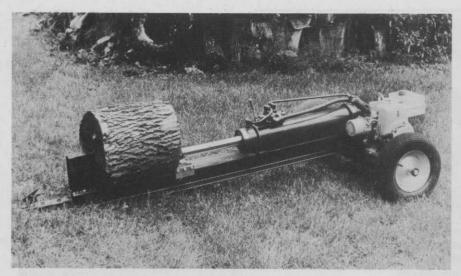
HYDRA-SPLITTER: This heavy-duty unit is designed to give many years of reliable, trouble-free service, says Didier Manufacturing Co. The unit exerts 10 tons of ram pressure with a 7 in. cutting wedge. It has a 20 second recycle time, powered by a 4 HP gasoline engine. This unit is also available in a PTO-operated model. Didier claims it will operate off any forklift, skid steer loader, or tractor with a three-point hitch.
