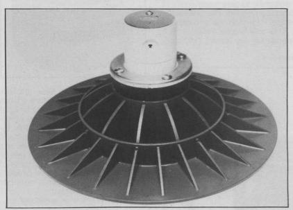
SUPPORT: A stabilizing support flange for irrigation sprinkler heads, is engineered and designed to be completely under the turf surface, says Sage-T-Lawn, Inc. The flanges protect heads from tilting or being pushed into the ground by heavy maintenance equipment. Drain holes in flanges prevent puddling around sprinkler heads.
