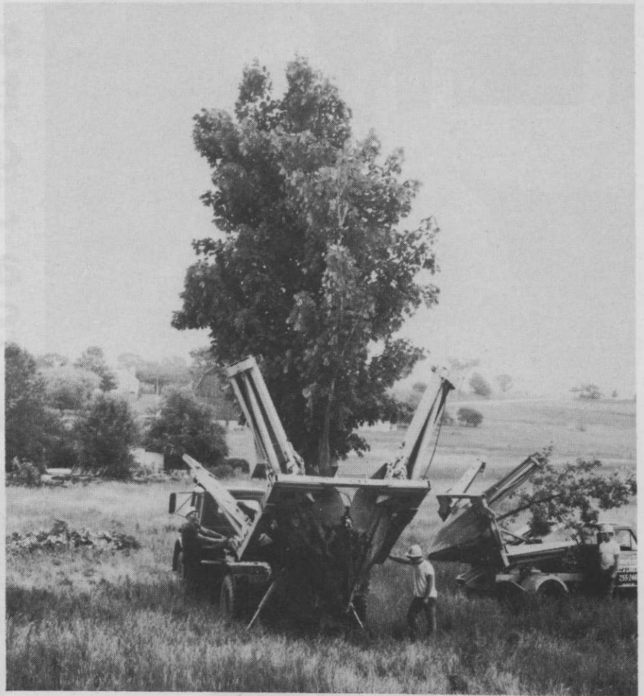
A major advantage of having a tree spade is the capability to perform special planting assignments quickly and cheaply. An instant mini-park or transplanting a donated specimen tree rose to a bicentennial rose bed can be completed with a minimum effort.
