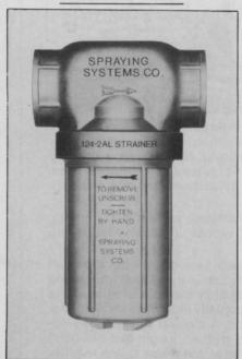
**STRAINERS:** Two new line strainers from Spraying Systems Co. feature a "threaded" bowl for quick removal and cleaning of internal mesh screen. Bowl can be rotated by hand for removal and replacement, with lugs on bottom of bowl to assist in operation. The 124-2 Line Strainers are supplied with 2 inch NPT(F) connections. 124-2½ Line Strainer has 2½ inch NPT(F) connections. Strainer heads are available in aluminum and cast iron with stainless steel screens. Bowls are made of glass-
