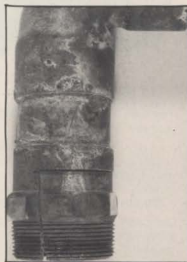
This is the two-inch ips male thread-to-tubing nipple soldered to a piece of two-inch tubing, in turn soldered to a two-inch to one and one-half inch reducing bushing, soldered to a piece of one and one-half inch tubing.
