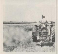
Century's powerful Mist Blower/Sprayer is 4 sprayers in 1, Blower rotates through a 210° arc. 3-point mounted unit equipped with 25-gal. ''Poly'' tank. Includes sturdy, trigger-type, brass 2-ft. handgun with 25 foot hose. Also has brackets for boom or jet spraying. Delivers 150-mph mist with swath up to 150 feet.
