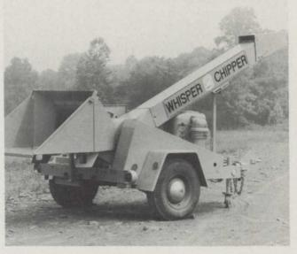
WHISPER CHIPPER: Over the past 25 years Asplundh has improved and redesigned their basic chipper, based on the direct reports of actual operators within their organization. Asplundh features four chipper models ranging from a 12-inch, 4 cylinder standard chipper to a heavy duty 16-inch, V-8 engine. The company claims the model 12-inch, 4 cylinder JEY has a reading of approximately 73 to 77 decibels at 50 feet. Other models vary, and noise level while chipping depends on material being chipped.
