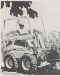
SKID STEER PAY LOADER: New from International Harvester is this 37 HP model. Unit is highly maneuverable with lift capacity of 1,950 pounds; has two-lever skid steering that permits 360 degree turns; hydrostatic drive with infinitely variable forward and reverse speeds from 0 to 8 mph; four-wheel drive; oscillating axles for better traction; changeable tread widths with reversible wheels; fast cycling loader; roll-over protective structure; and a variety of quick-change attachments.
