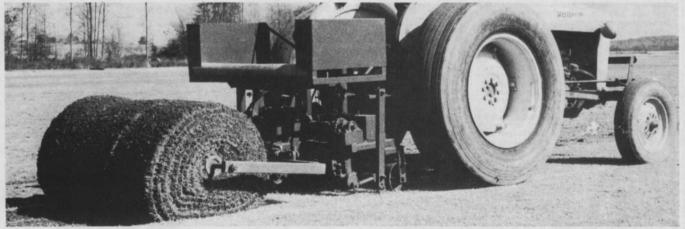
Three or four men can cut and roll 1200 yards of sod an hour with this machine, according to its manufacturer. It is the Beck Sod-o-Matic, a harvester which brings sod into large rolls, 3-16" strips 45 feet long, 180 square feet, 20 square yards. The big roll is started around either cardboard tubes or other type tubes and, when completed, can be moved and loaded by fork lift. At a job site, the big rolls are unloaded by and picked up by the tractor equipped with a laying device.
