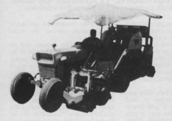
The Nunes Mechanical Sod Harvester features hydraulic controls which the manufacturer says allow for quick and easy adjustment to different field, terrain, soil and sod conditions while the unit is in operation. The unit, Nunes says, will cut, lift roll (or slab) and palletize more than 1000 square yards of sod per hour. The unit handles either rolls or slabs 12 to 20 inches wide (24-inch width machines on special order).
