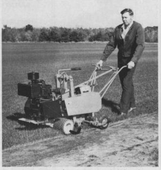
This is the Ryan Heavy Duty Sod Cutter, which through conversion can cut 12", 16" or 18" wide. The manufacturer says one man can cut 14 to 14 acres of sod per day. The cut-off model offers automatic, vertical cut-off adjustable from 1 to 9 feet. There are two propulsion speeds on all models. The drive to the eccentric is now through heavy-duty spur gears. There's also an improved belt drive, the manufacturer says. A sulky roller attachment is available.
