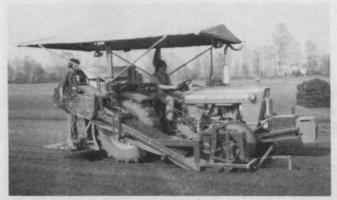
The Brouwer Sod Harvester, its manufacturer says, will produce up to 1300 square yards of sod per hour with 2-3 people. The unit will roll, slab or fold sod and is built to cut in one of four widths: 15", 16", 18" or 24". Designed to mount on either a Ford or Massey Ferguson standard farm tractor, the Brouwer unit's most recent development is a 3-inch blade. The "throw away" side blades and bottom blade, the manufacturer says, are less expensive than conventional blades.
