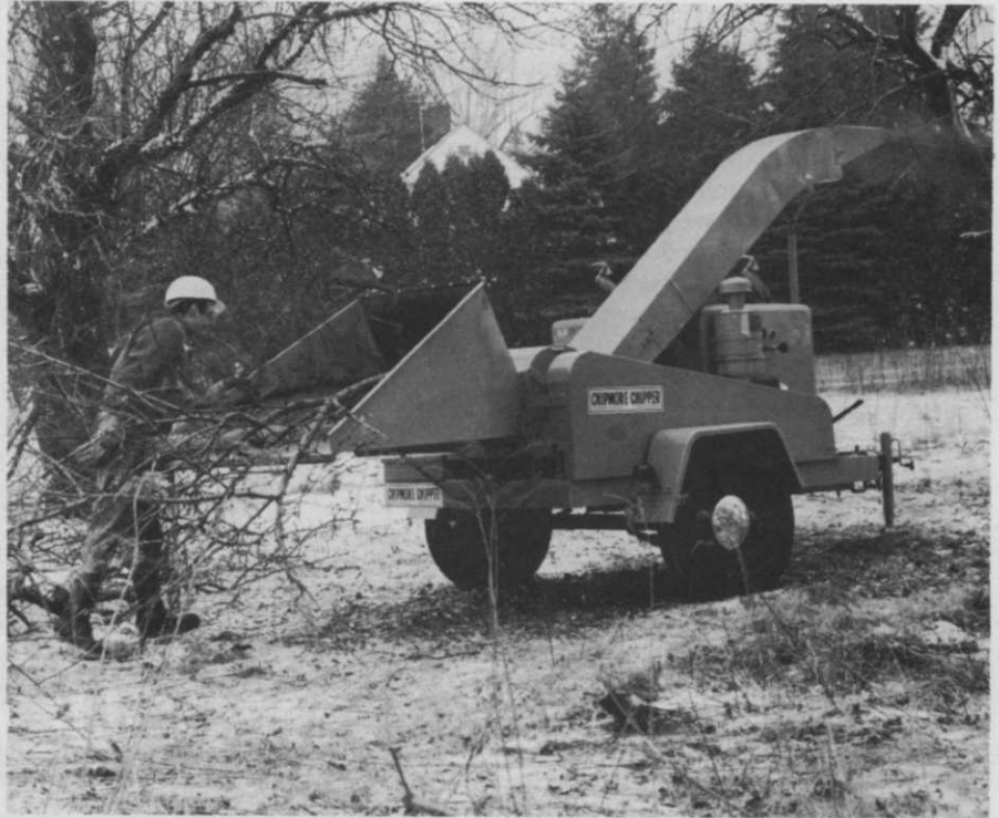
A chipper can, conservatively, reduce five to eight truckloads of brush and branches to one truckload of chips; free as many as four men for other work assignments; provide a good bio-degradable substance for soil structuring, weed control, ground cover and mulch. But purchasing an over-or-under-powered unit or one not heavy duty enough for your type of work can result in just as many negative aspects.
