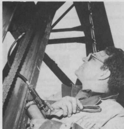
A rough terrain forklift needs its own brand of tender loving care. Some of this care includes frequent cleaning and lubricating of the mast chain.
