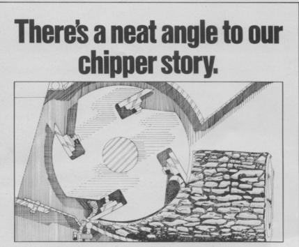
The secret's in the rotor. Being a steel forging, rather than a vulnerable casting, it has the structural strength to permit the blades to be positioned at the precise angle for slicing. No more chopping and mangling wood. Or spending an hour or two adjusting rotor blades. Our positive V-lock design reduces adjustment time to a matter of minutes.
