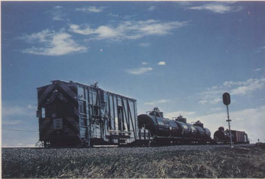
Spray trains are efficient on mainlines in wide-open territory where it is possible to spray over 100 miles per day.
