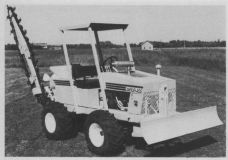
DIGZ-ALL: This unit is equipped with a 37 HP Wisconsin VG4D engine. It is built primarily for heavy-duty trenching, says the manufacturer. ROPS and fully hydraulic backfill blade are standard components. Ground drive for trenching is infinitely variable and hydraulic. Trenching depth range is from 40 in. to 82 in. with a range of 5 in. to 18 in. trench width. Digging speed is 0 to 30 fpm.
