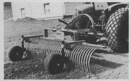
RAKE: York Rakes introduces this new unit designed and built specifically for use with the new 20 to 30 HP tractors. Up until now, according to the manufacturer, landscapers using this new breed of tractor had to resort to rakes built for other horsepower ranges. This unit features welded steel construction and a seven foot working width. The rake can be drawn straight across for leveling and spreading soil, or can be angled to the right or left to discharge excess soil, rocks and debris.
