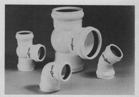
FITTINGS: Lasco Industries introduces these new gasketed pressure fittings for water distribution and irrigation systems. Extra-depth sockets in the fittings maintain integrity of the seal and compensate for earth movement, uneven trenches, expansion and contraction of the pipe, as well as lateral movement, says the manufacturer. These units use the supremacy of a sphere as the strongest shape for a pressure container.
