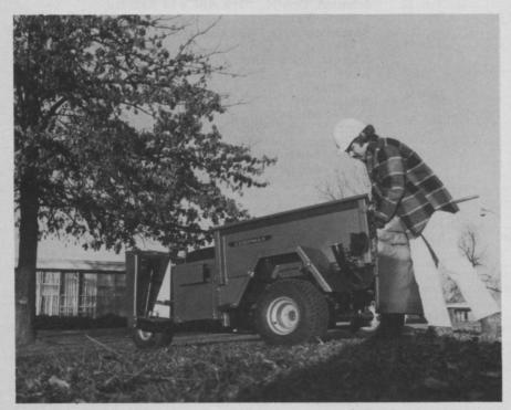
NEW FEATURES: Automotive steering and shock absorbers are new standard features on 1976 model Cushman Runabout vehicles. Other standard features on the three-wheel utility cart include turf tires, front shocks and a utility pickup box measuring 46 in. x 34¾ in. x 14 in. Equipment options include front bumper, speedometer, overload springs, steel cab with cloth or steel doors and an exhaust spark arrestor set.
