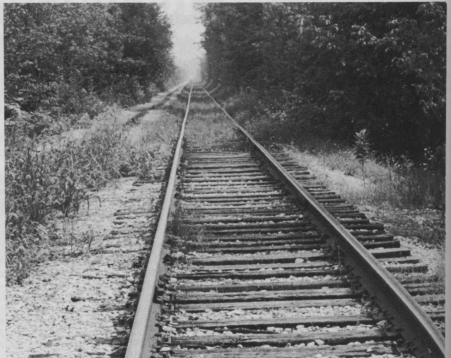
Foreground shows the results of an herbicide application made in May, 1975, compared to check area.
