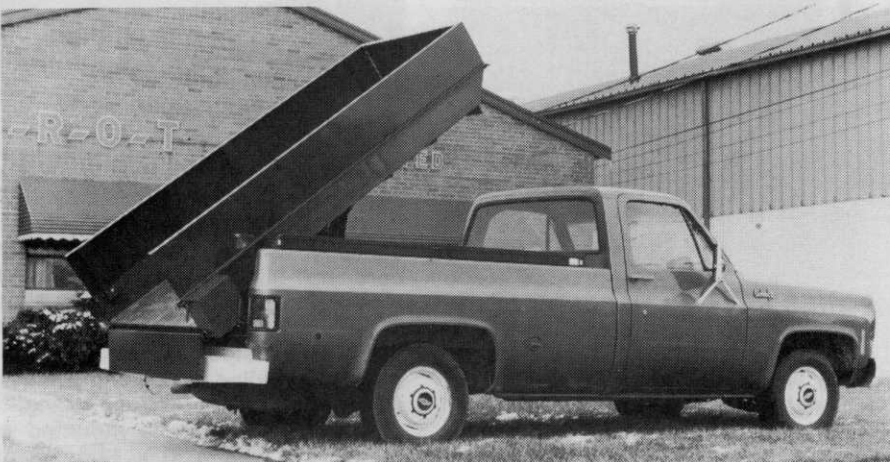
JIFFY DUMPER: This unit, from B.R.O.T. Incorporated, has a self-contained hydraulic lift and fits pickups, fleetside or stepside (Ford, Chevy, Dodge, International). It is called the Jiffy Dumper, able to dump up to 3,000 lbs.
