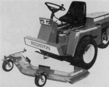
THREE WHEELERS: Hesston has the new Front Runner Three Wheeler, available in either a 16 hp or a 19.8 hp model. It has a heavy-duty automotive gear box with rack and pinion steering. Front-wheel hydrostatic drive and high-flotation turf tires are meant to give stability and traction. The manufacturer says one lever controls instant forward/reverse and infinitely variable speeds from 0 to 11 mph in either direction with no gears to shift.
