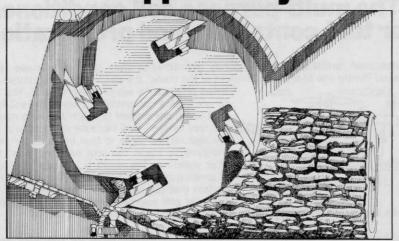
The secret's in the rotor. Being a steel forging, rather than a vulnerable casting, it has the structural strength to permit the blades to be positioned at the precise angle for slicing. No more chopping and mangling wood. Or spending an hour or two adjusting rotor blades. Our positive V-lock design reduces adjustment time to a matter of minutes.
