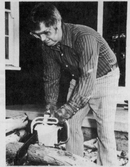
CHAIN BRAKE: McCulloch's Mini Mac 25 chain saw is now equipped with a chain brake to help reduce the hazard from "kickback".
