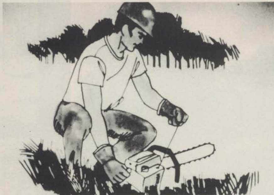
Steady the saw, keep your balance and start the saw on the ground or other solid surface.
