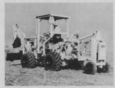
Both of "The Diggin' Dutchman's" M-440 (with liquid-cooled engine) and M-437 (air-cooled) machines feature P-12A vibratory plows with quick-tar-h reel carrier.
