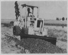
At the same time, you double your job capacity with a backfill blade that swings 45° left or right and tilts hydraulically for sloping surfaces
