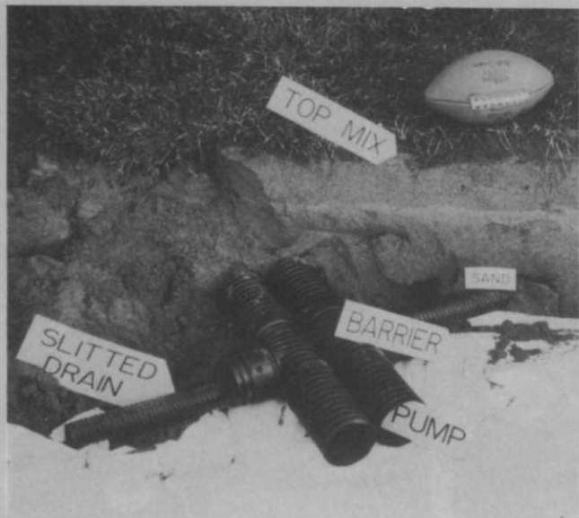
This profile model of a PAT system shows the plastic barrier, collector pipes and slitted drains.
