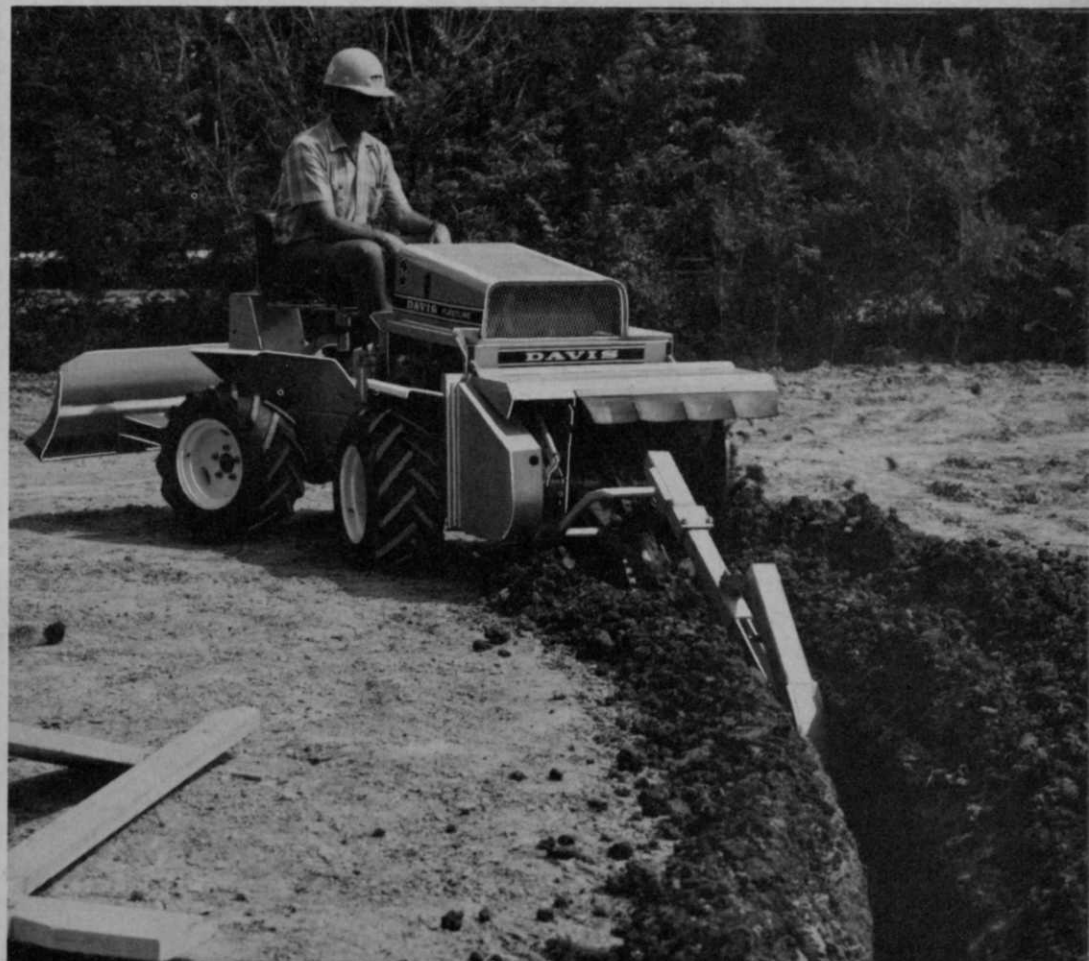
SP-40 direct-burial Line-Layer buries line, cable and flexible tubing to 24" deep.
