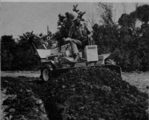
Fully hydraulic backfill blade offsets to counter side thrust. Operator has direct-line vision to the job.
