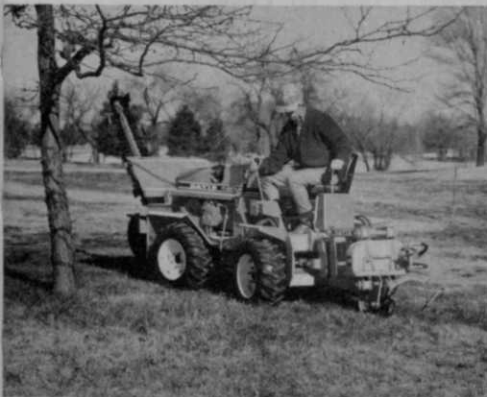
SP-40 direct-burial Line-Layer buries line, cable and flexible tubing to 24" deep.
