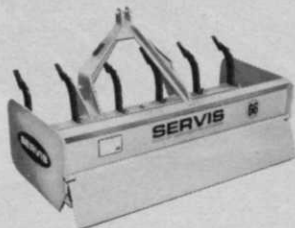
SECO, JR. models (66" and 72") are popular with operators who do not usually require scarifier teeth for their routine work. Optional teeth can be positioned manually in UP or DOWN position.
