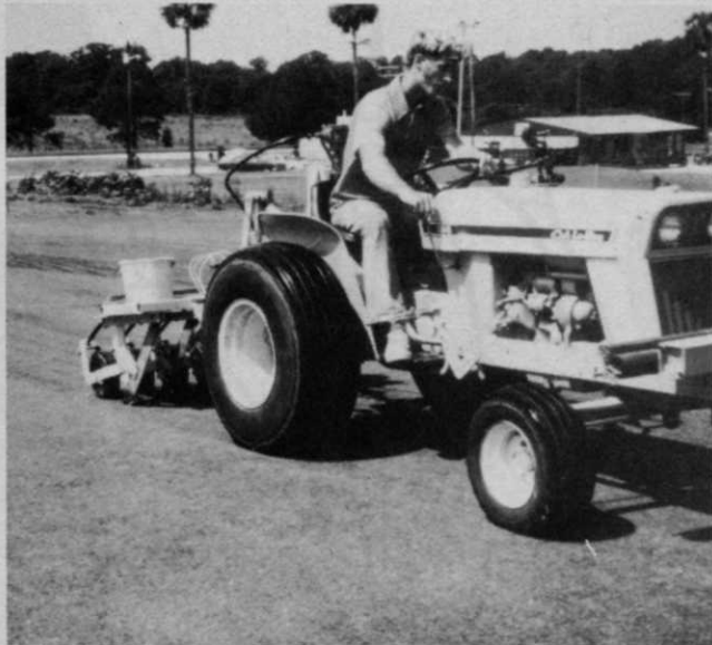
John Russell, son of owner, operates the greens model fumigating rig. It is smaller than the fairway model rig developed about three years ago.
