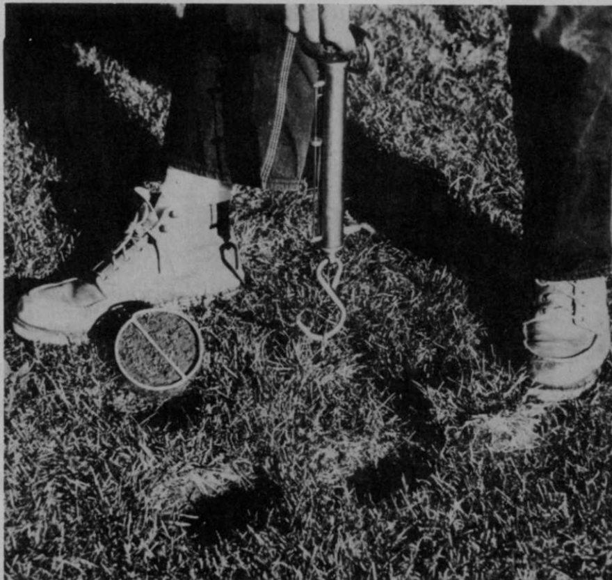
A sod plug is pulled from the soil to measure the force necessary to separate it from the soil. The metal hook is inserted through a nail hole and attached to the cross bar. A scale attached to the other end of the hook measures the maximum force necessary to lift the plug.
