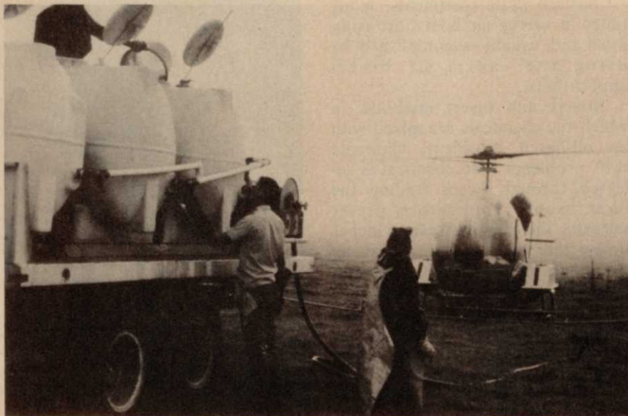
A nurse truck, loaded with premixed chemical, is used for tank refill on one of Southeastern Helicopter Service's choppers. The truck follows landward as the aircraft treats the weed-choked canals.
