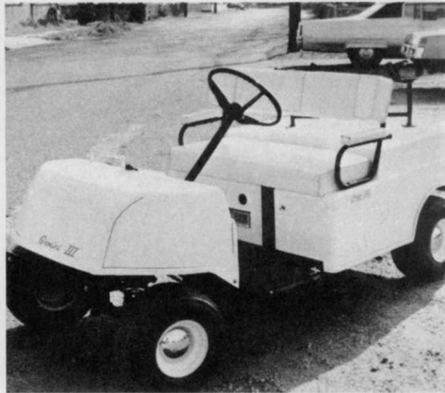
PROPANE-POWERED GOLF CAR: Model Tee Cart Corp. Keyport, N.J.
