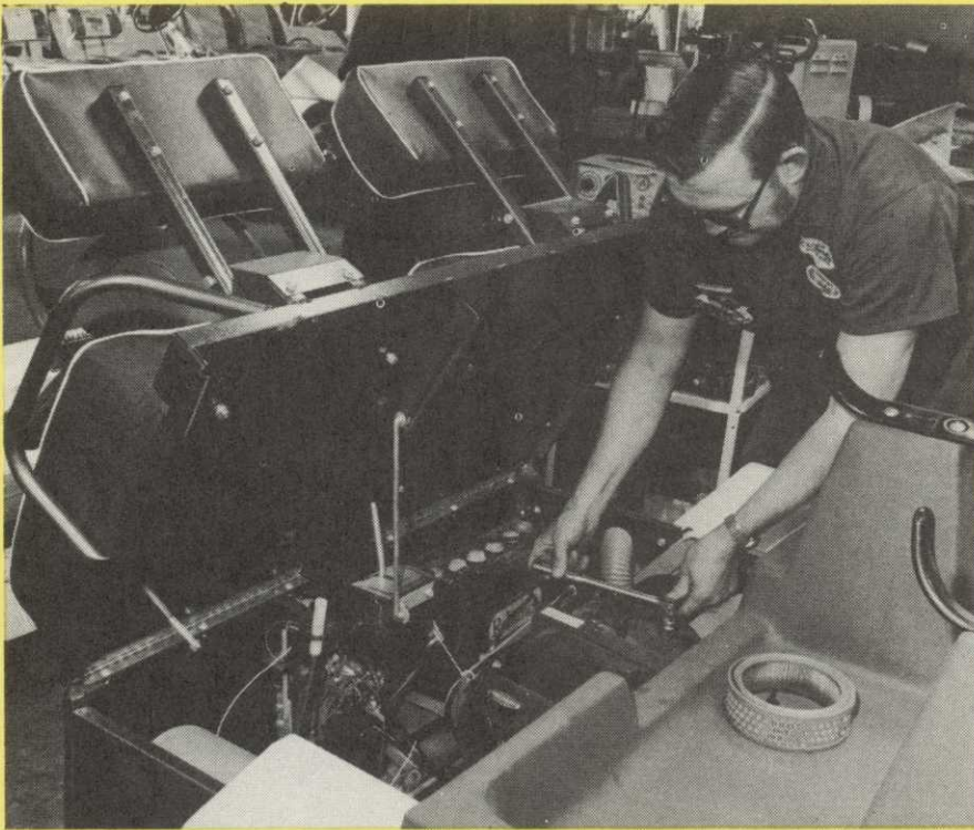
Small engine maintenance is not difficult. It does require regular checks on vital parts. Here workman checks engine and replaces air cleaner.
