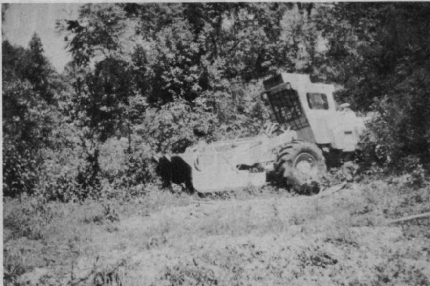
This gigantic brush chopper built by National Hydro-Ax can clear brush at a cost of about $64 per acre. This compares favorably with other methods of brush control along utility rights-of-ways.
