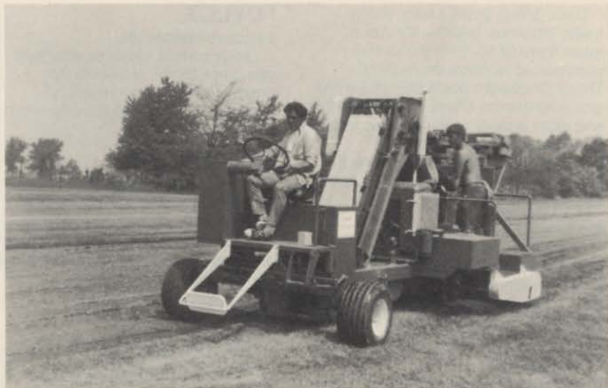
Princeton Manufacturing Company builds three basic models of sod harvesters which cut and palletize sod in one operation. The most recently developed model is designed with maximum flotation to permit operation in extremely soft conditions.
