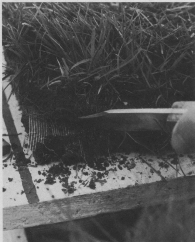
Plastic netting functions as a reinforcing member in a sod sample. Some six-month-old sod was tested to a pull strength of 200 pounds when grown with netting.
