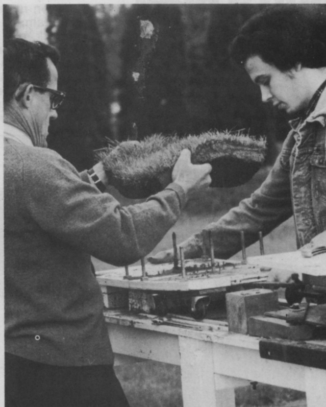
Dr. William Mitchell (left), extension agronomist at the University of Delaware, places netting-reinforced sod on a machine designed to test the pull strength of sod.
