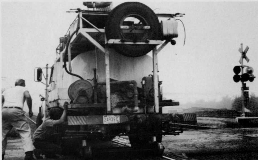
The on-off the track vehicle applies about 25 to 30 gallons per acre. In addition to being more economical than spray trains, they are more efficient and result in fewer claim damages.
