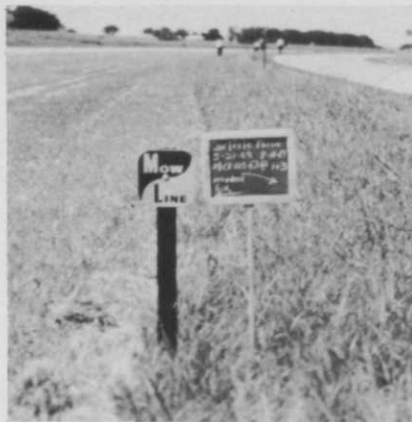
Highway median left of sign was mowed six times. Grass on right was mowed once, representing a savings in maintenance costs.
