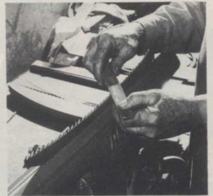
Use a large flat file to joint curved pruning saws. Usually one or two strokes across the tips of the teeth running the blade length will do it.
