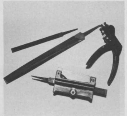
Here's the tools you need to sharpen your own saws: a six-inch Cant saw file, large flat file for jointing, pistol-grip saw set tool, and jointing tool for straight blades.
