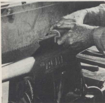
For straight saw blades, use a jointing tool. Note how saw blade is securely held in the vice so it won't wiggle or come loose.
