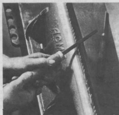
This man has been making and filing saws for 35 years. Note how he holds file. Saw vice holds saw firmly leaving blade exposed.
