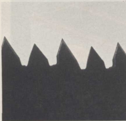
This is a typical saw that needs to be sharpened. Notice how the teeth are uneven in height and bevelled wrongly. It does not cut cleanly or smoothly.
