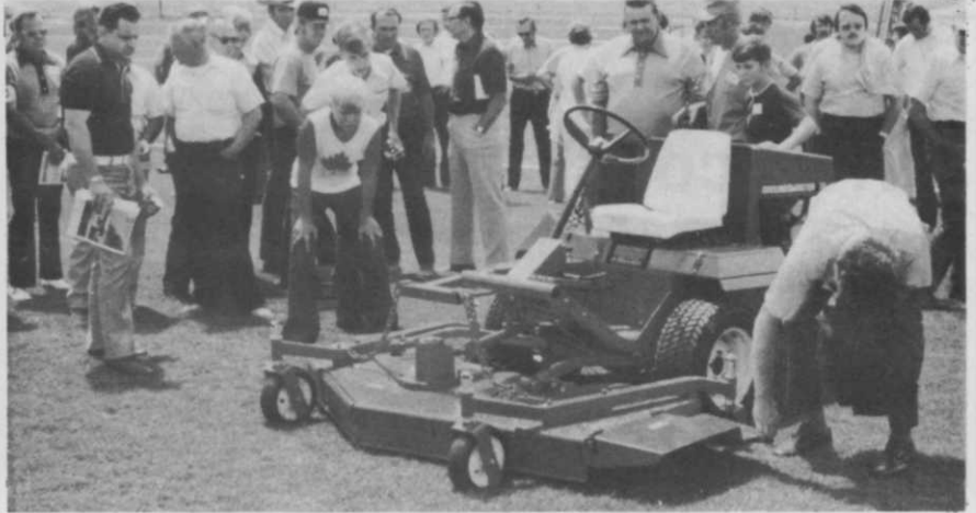
This Toro Groundsmaster 72 mows a swath 72 inches wide. Mower height is adjustable front and rear from 1/2-inch to 6 inches. It was one of several mowers demonstrated by the company during the field day.
