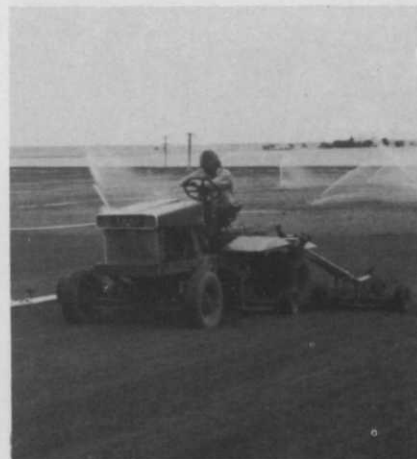
This Parkmaster has nine gangs. All are hydraulically operated by controls easily accessible to the driver.
