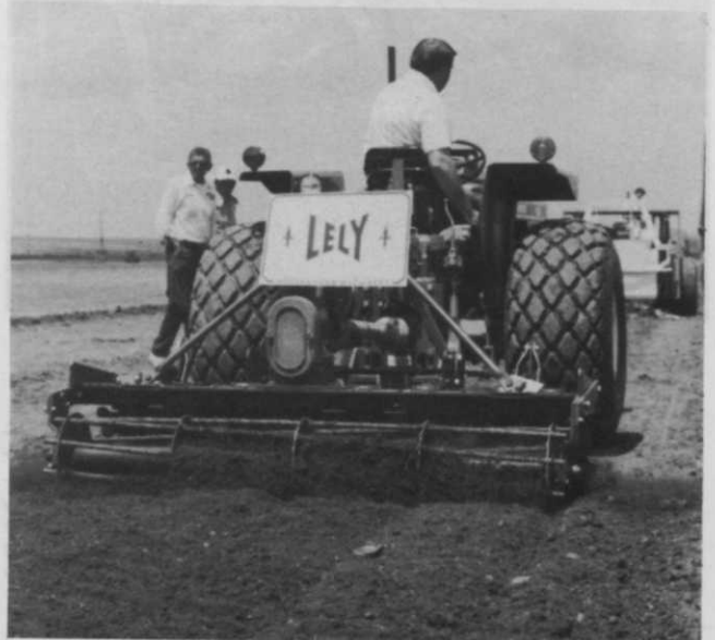
Roterra, a power-driven rotary harrow, pulverized dirt into a smooth seedbed. It's made by Lely. Vertical tines in the front of the unit whirl through the soil with an "eggbeater" action. It's mounted on a 3-point system and PTO driven.
