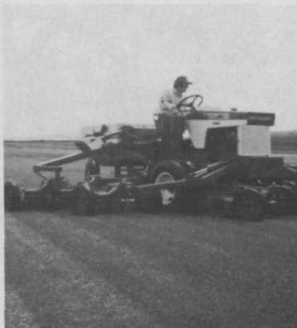
Model F20 of the Jacobsen turf tractor quickly mowed the demonstration area with ease.
