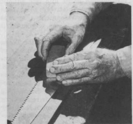
A final saw tip. Lay saw on flat surface. Run a honing stone down the saw blade to take off metal burrs. It will put a professional touch to your work.
