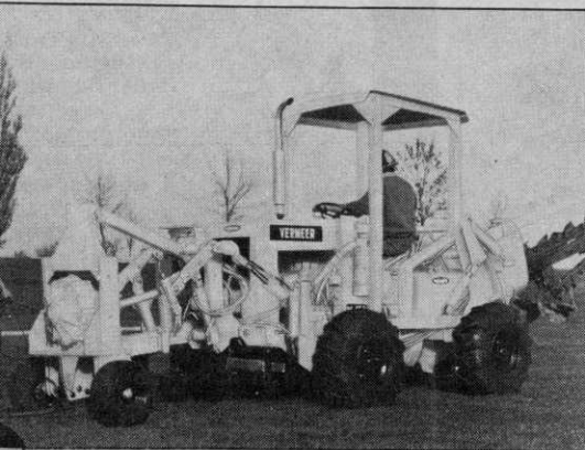
Front-mounted P-20 Plow on Vermeer M-465—Four-wheel drive, center-pivot articulation . . . Trailer-type design isolates vibrating action from drive unit for positive underground installation. Dual lift and tilt cylinders control blade angle.
