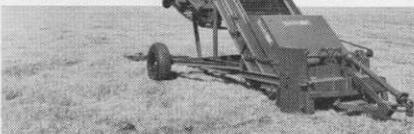
Designed especially for Custom operators. Digs, loads and cuts to planting length 1000-1200 bu. of clean sprigs per hr. . . up to 2000 bu. when equipped with Side-Loading Elevator. Floating PTO Shaft and Shear-Pin protection. Heavy-duty construction.
