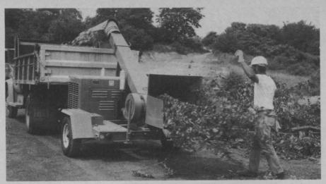
From tree limbs to wood chips. That's what West Mifflin, Pa. street commissioner Francis J. Horn is doing with branches from trimming jobs. He gives the chips to the citizens for use as mulch. Previously, brush was burned. Horn uses this M-B Chipper because it has no flywheel, instead, a spring-supported feed plate that adjusts to various wood sizes.
