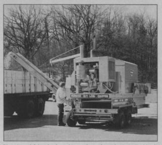
It's automatic! Just load any log or piece of wood-up to 4' wide, 6' long-into the hopper... where carbide-tipped cutting teeth chew it to chips in minutes. Handy conveyor then deposits chips in truck for easy disoeal.
