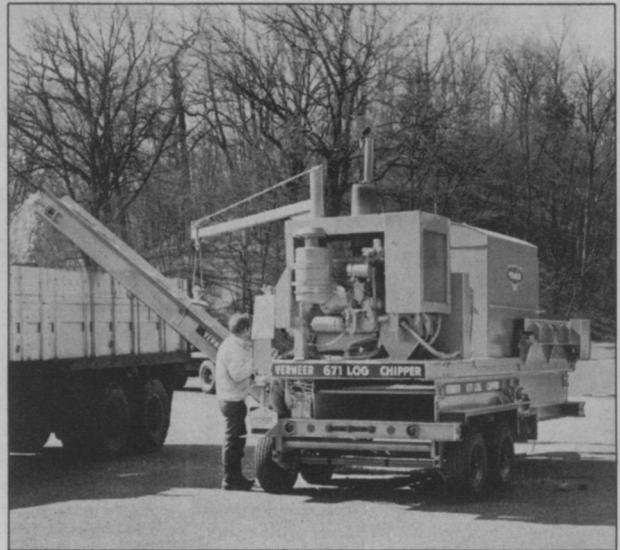
It's automatic! Just load any log or piece of wood—up to 4' wide, 6' long—into the hopper... where carbide-tipped cutting teeth chew it to chips in minutes. Handy conveyor then deposits chips in truck for easy disposal.
