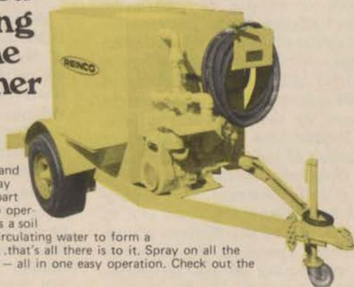
One man can easily fertilize, seed, and mulch up to 6 good size lawns a day with the PP500. Only one moving part insures low maintenance. Simple to operate. Add mulch, seed, fertilizer plus a soil binder such as Terra Tack to the circulating water to form a homogenous slurry. . . then spray. . . that's all there is to it. Spray on all the ingredients necessary for good turf - all in one easy operation. Check out the time. . . you'll be surprised.
