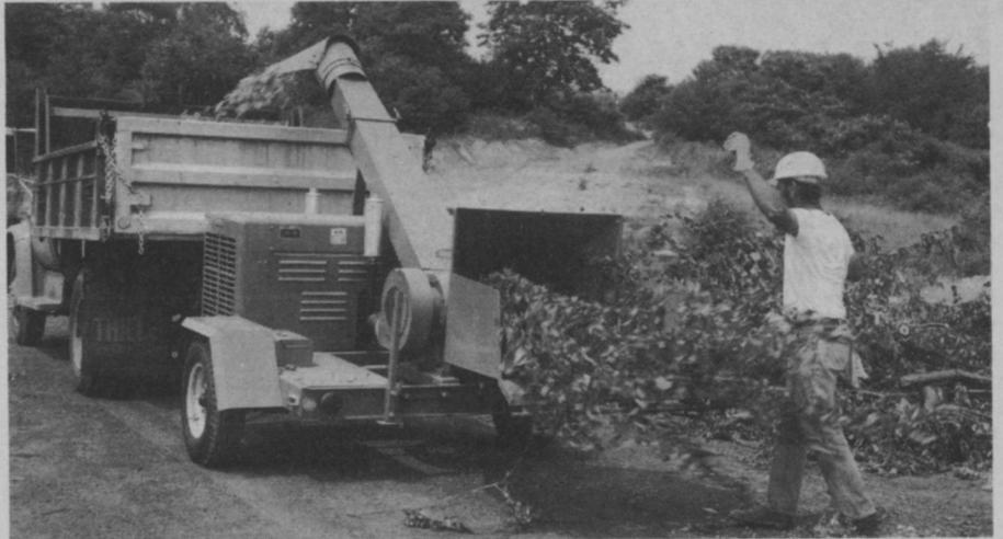
From tree limbs to wood chips. That's what West Mifflin, Pa. street commissioner Francis J. Horn is doing with branches from trimming jobs. He gives the chips to the citizens for use as mulch. Previously, brush was burned. Horn uses this M-B Chipper because it has no flywheel, instead, a spring-supported feed plate that adjusts to various wood sizes.
