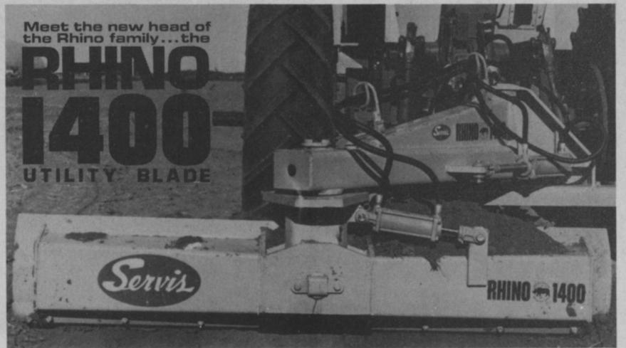
Designed for Category II and III tractors of 90 hp and up, this new leader of the Servis RHINO family puts more than 1400 pounds of mass into every ditching, grading, and backfilling job. Optional hydraulics control (at a touch) the patented main frame rotation and blade tilt. The RHINO 1400 has an eight foot moldboard, and support stand for hitching. Adaptable for quick-coupler.
