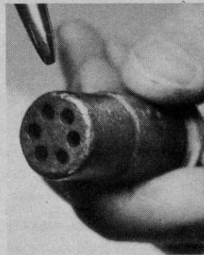
This nozzle tip can spray a stream up to 80 ft.
