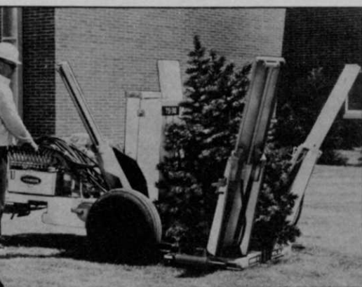
TS-30 Tree Spade—Ideal for hard-to-reach tree moving operations. Spade assembly angles in either direction for "tight quarter" maneuvering. Digs maximum tree ball 30" in diameter, 26" deep. Tows easily behind small truck or tractor.
