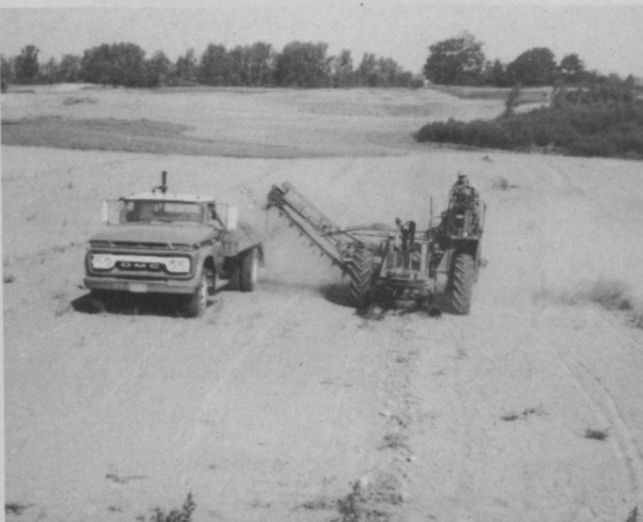
Stones are windrowed for easy pickup. When finished the course is ready to seed. Bergman picks up stones as small as three-fourths inch. Picker works on most any terrain.
