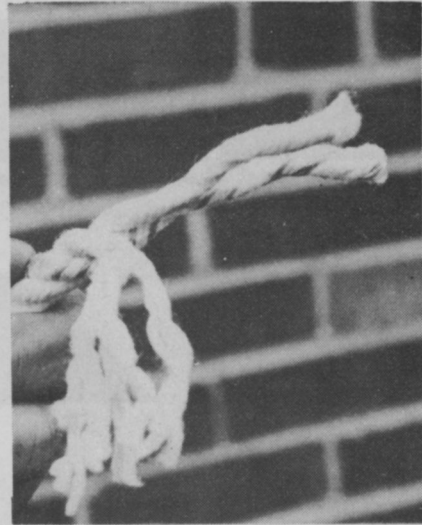
This is Esterlon polyester rope. Note the frayed strands. They tend to stay together to form a tight bundle of fibers. Color is lighter than manila.
