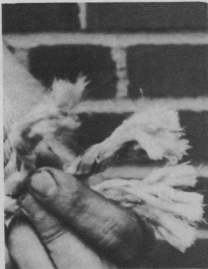
Manila rope is composed of fibrous strands that can break or become worn. Safety lines should be inspected daily and stored properly at night.
