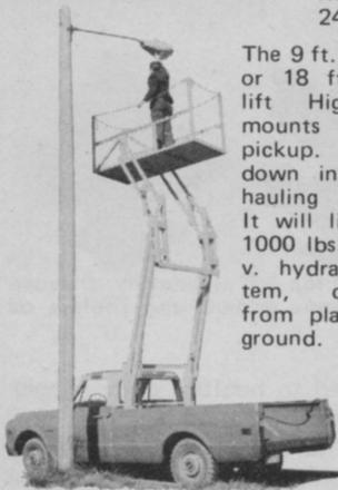
The 9 ft. single lift or 18 ft. double lift High-Worker mounts in any pickup. Folds down in bed for hauling materials. It will lift up to 1000 lbs. with 12 v. hydraulic system, controlled from platform or ground.
