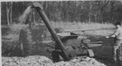
Chips limbs up to 4" diameter. Now has longer, wider feed chute, improved feed roll, blower and chute assembly. Standard hammer-mill rotor. Optional hopper permits processing soil, leaves, stalks, hay or bark. PTO and gas engine drive models. Check coupon for details.
