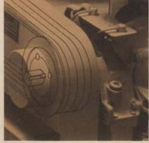
Optional torque converter isolates engine and transmission from cutting shock to minimize maintenance. Makes operation virtually fully automatic; increases operator productive time. Available on all models.
